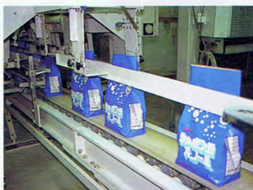
Soap powder is bagged on a conveyor to produce soap packages for laundry.
